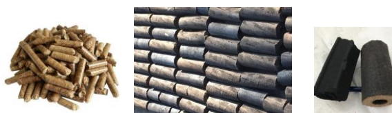
Bamboo pellets (left); bamboo briquettes (middle); and bamboo charcoal and torrified (right). Photos downloaded from the company's website.
